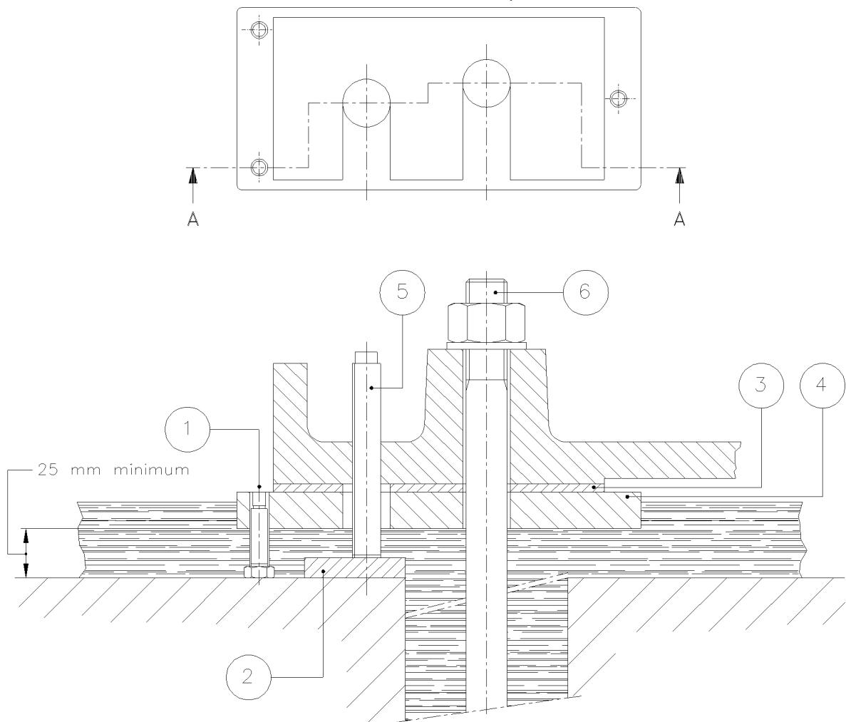
1. Sole plate positioning bolt
